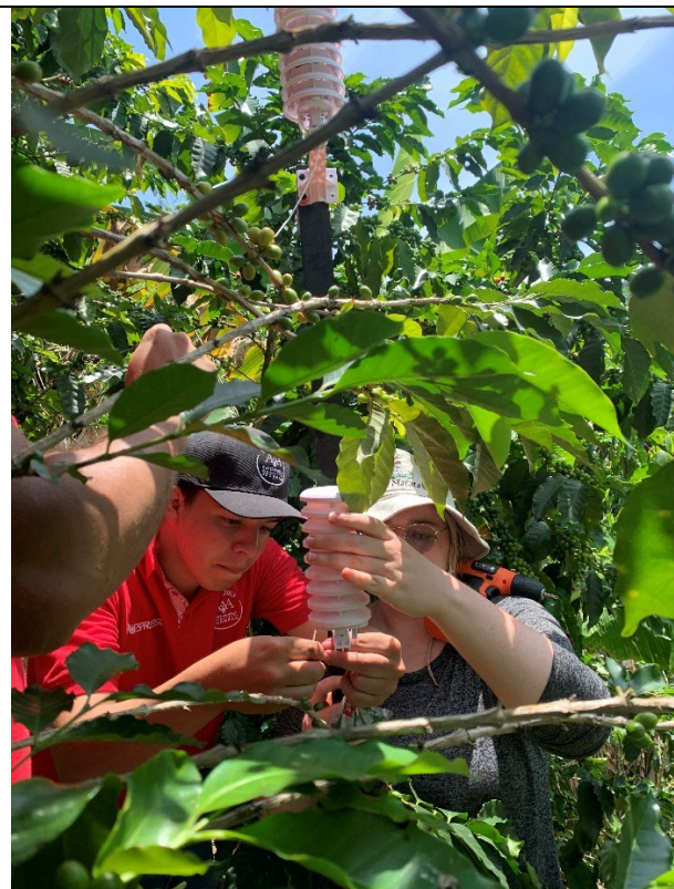
Figure 1. Farm set-up: installation of temperature loggers (+ radiation shields) by project staff on each farm
